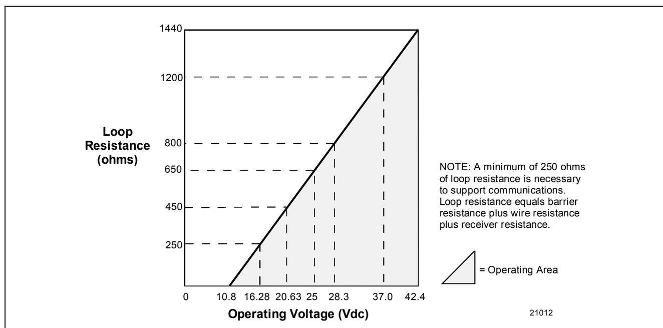
**Figure 2** —Supply voltage and loop resistance chart.
