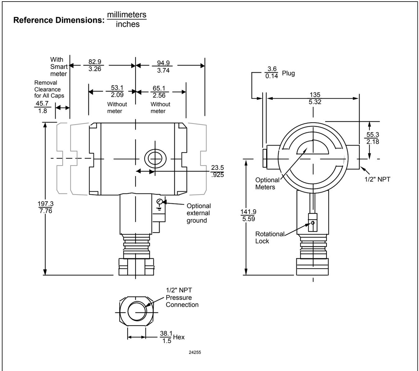
**Figure 6** —Typical model STG90L mounting dimensions for reference.
