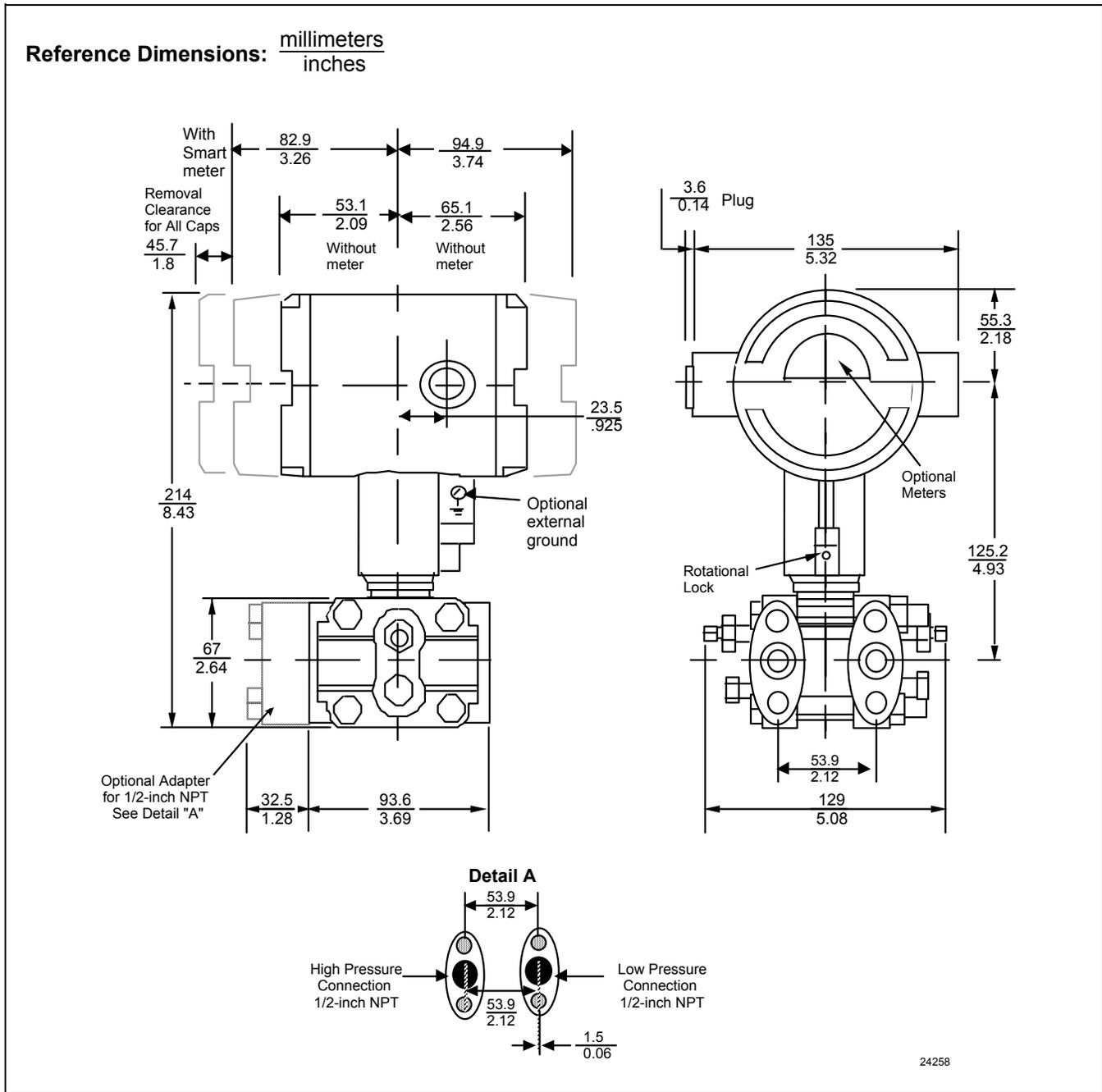
Figure 5 — Typical model STD904 mounting dimensions for reference.
